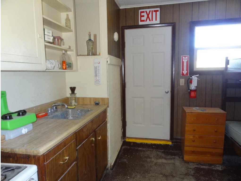
S.C. Rearing Station Office & Garage - Building #0666 Description: Exit sign and egress lighting installation needed.
