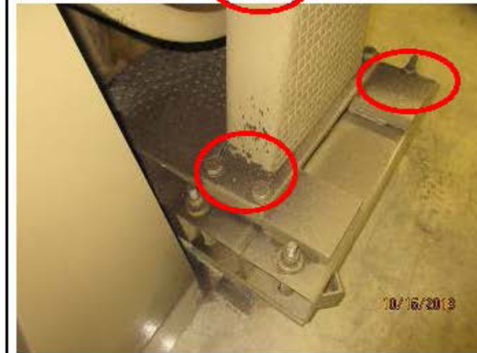
Ropes showing wear. Rope debris.
